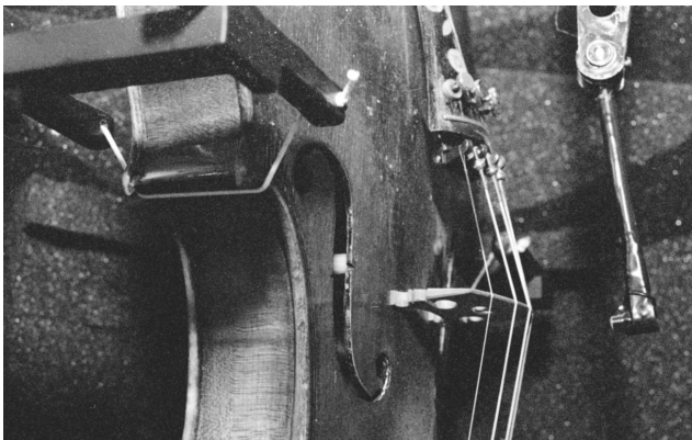
Fig. 1: Support fixture with low mass, low damping, flexible support elastics placed close to hammer strike axis to minimize torque, and subsequent rigid body rotations
