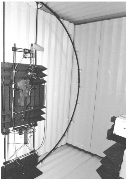
Fig. 2: Automated normal mode vibration and acoustical measurements system for violin, inside anechoic chamber
