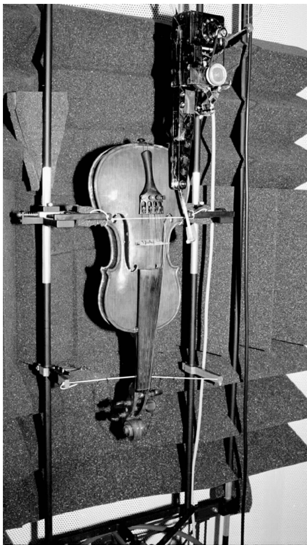
Fig. 1: Treble violin mounted in free-free, zero-mass loading modal analysis configuration (force hammer excitation, scanning laser response)
