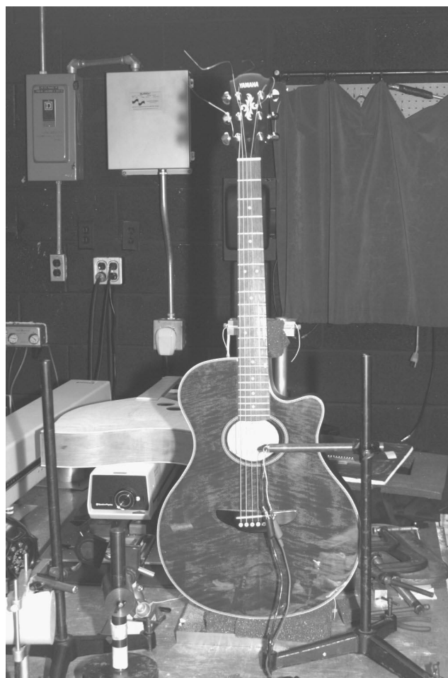
Fig. 2: A folk guitar undergoing vibrometer testing to determine string response
