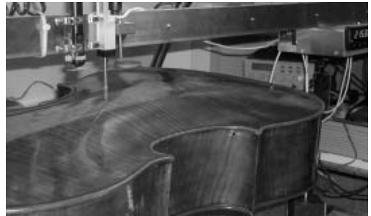
Figure 1. Device for measuring arching profiles on an X-Y coordinate table.
