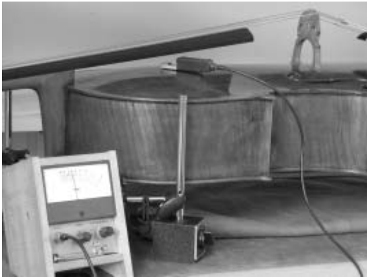
Figure 3. Device (prototype) for measuring the thickness graduation. The thicknesses are shown on the analog scale and processed by a computer to calculate the interpolation maps ( Instrument: Cello by Domenico Montagnana, 1740 ).
