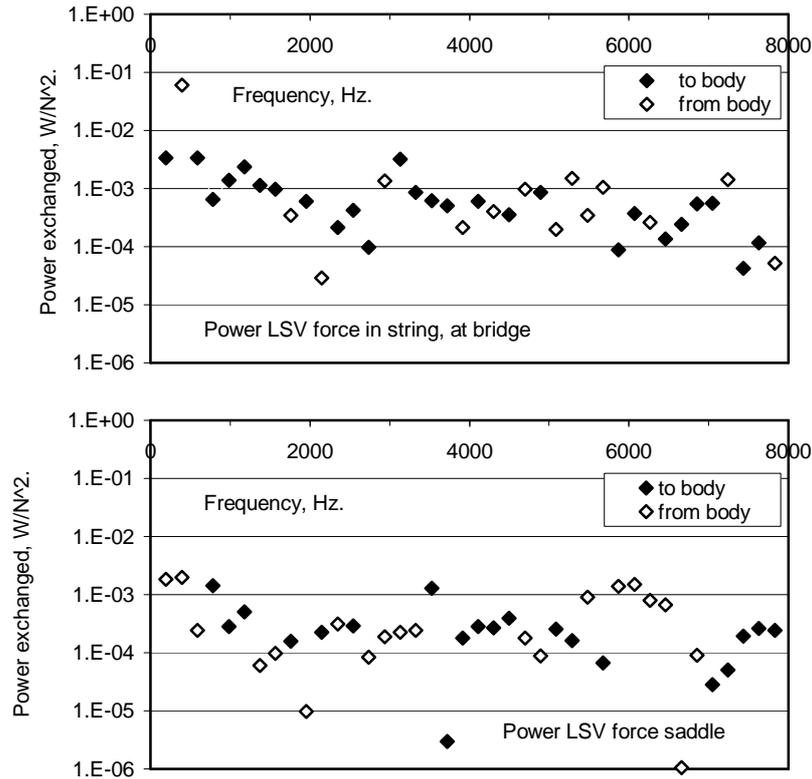
**Figure 3. The power in Watts exchanged per unit force squared. Shown for a TSV force and an LSV force at the bridge, and for an LSV force at the saddle. The data is presented at 196 Hz intervals only.**
