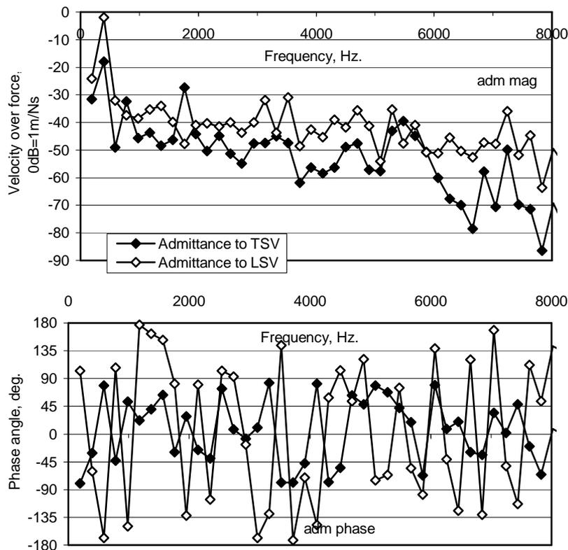
**Figure 2. The magnitude and phase of the pseudo-admittance of the bridge to the forces applied by a transversely vibrating string. The data was only found at 196Hz intervals and are shown as points. The points are joined by lines to improve the clarity of presentation.**
