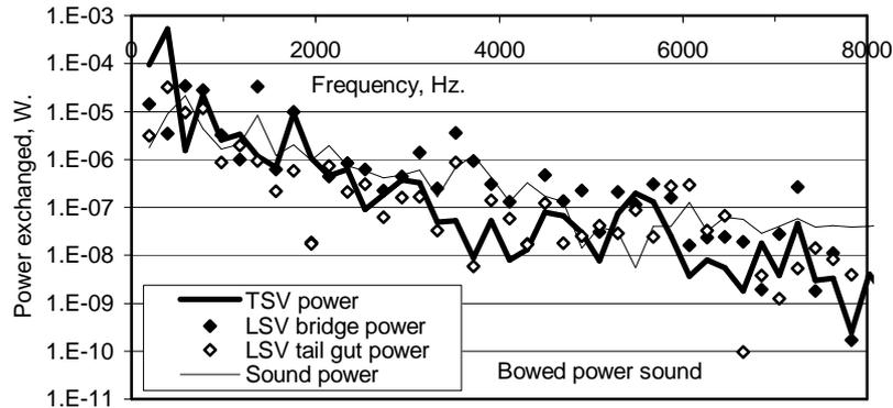
**Figure 4. Power input to the body by TSV at the bridge, compared with the power exchanged at the bridge and saddle by LSV (the TSV data points and the LSV direction of power transfer are omitted for clarity). The radiated sound power (uncalibrated, and arbitrarily positioned) is shown for comparison (data points omitted for clarity).**
